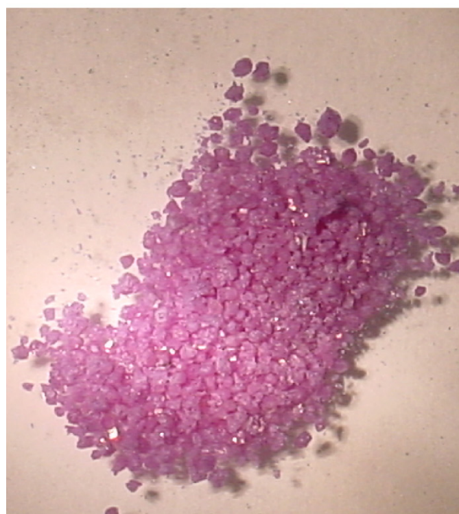
Fig. 7. Optical images of Nd_3Li_5Ta_2O_{12} crystals illuminated by: (a) a standard fluorescent light bulb and (b) a standard incandescent light bulb.
